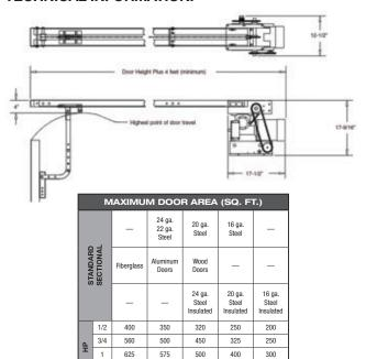
NOTE: On steel insulated doors, a 24-gauge back panel is assumed. If a heavier back panel is supplied, use the next higher HP rating. Recommended Duty Cycles: 25 per hour, in excess of 90 per day.
